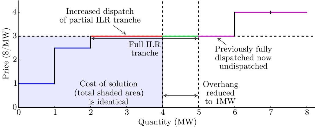
Figure 3: Example of reserve dispatch solution using intelligent selection.
