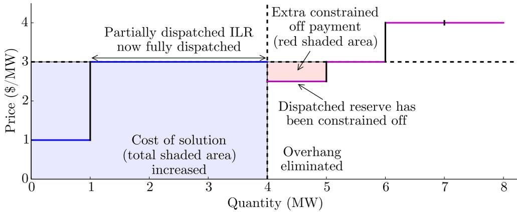
Figure 5: Example of reserve dispatch solution using constrained off payment.
