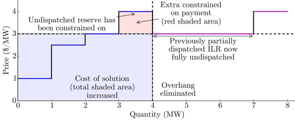
Figure 4: Example of reserve dispatch solution using constrained on payment.
