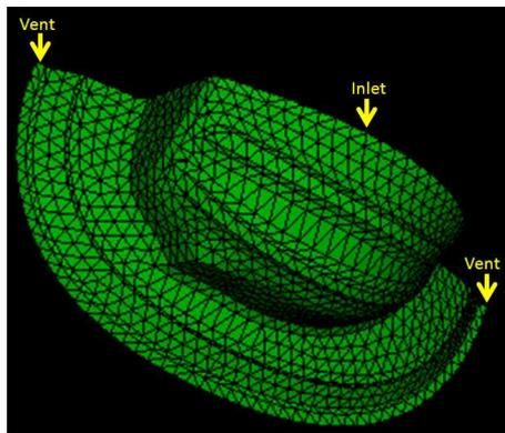
Figure 6: The medium mesh of a fireman's helmet.
