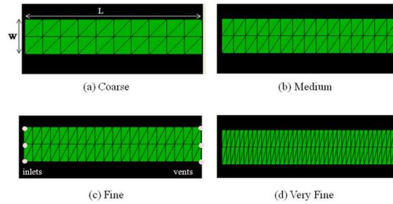
Figure 2: Four meshes for the flat rectangular plate model used in CRTM simulation.
