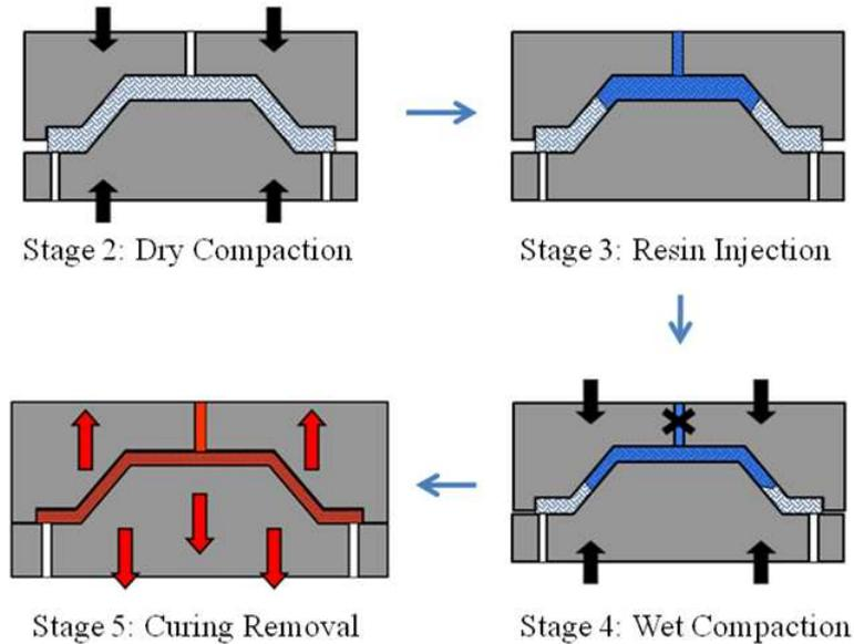
Figure 1: LCM process: Stages 3 to 5.
